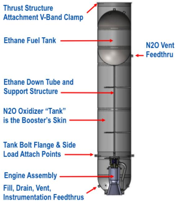
**Figure 4.0 MNMS Booster Cutaway**
