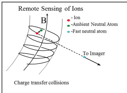
Figure 21: MINI-ME Concept of Operation
