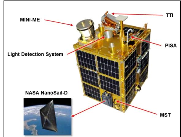
Figure 3: Six Instruments on FASTSAT-HSV01
