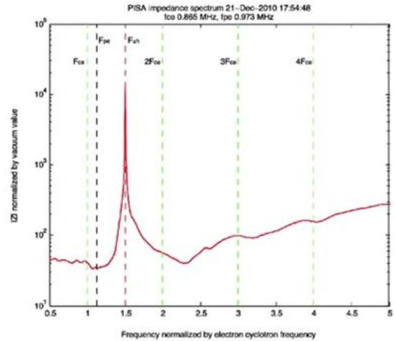
Figure 17: Single PISA Impedance Spectrum, Showing Resonance
