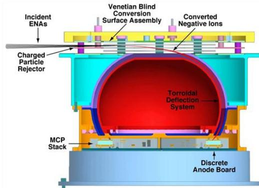
Figure 22: MINI-ME Instrument Configuration
