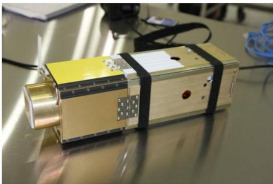
Figure 12: NanoSail-D 3U CubeSat Pre-encapsulation
