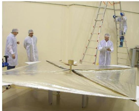
Figure 13: Ground Deployment Test of 10-m<sup>2</sup> Solar Sail
