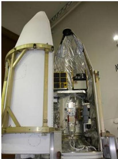
Fig. 2: Six Spacecraft Integrated on Minotaur IV at Kodiak Launch Complex
