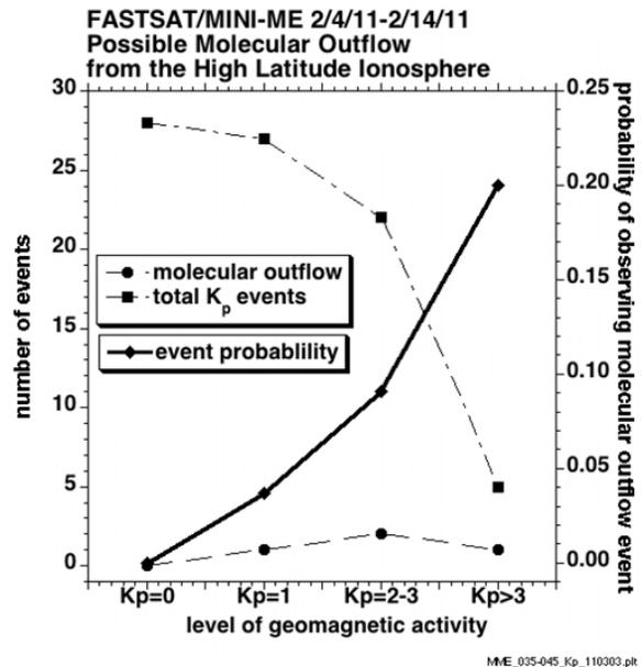
Figure 23: Possible Molecular Outflow from High Latitude Ionosphere
