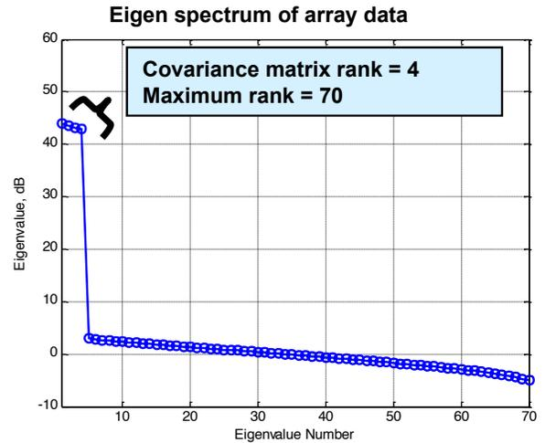
Figure 1. Eigenspectra of the jammer space-time covariance matrix used to form the data for the simulation. The small number of significant eigenvalues represents a sparse signal structure within the data, which is ideal for applying CS approaches to detection and estimation.
