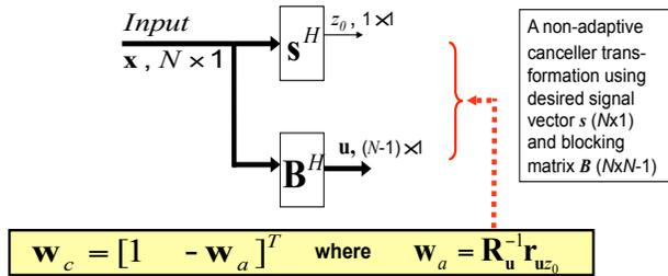
Figure 2. Generalized Sidelobe Canceller: GSC transformation and subsequent adaptive solution,  $\mathbf{w}_c$ . Superscript  $H$  denotes conjugate-transpose.
