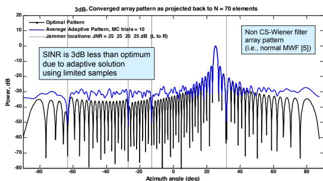
Figure 4. Adaptive (top) and optimal (lower) STAP antenna patterns. Adaptive pattern generated using MWF operated at a rank of five, and using  $2r = 10$  temporal samples. There are 70 spatial and 10 temporal samples, or 700 total samples.
