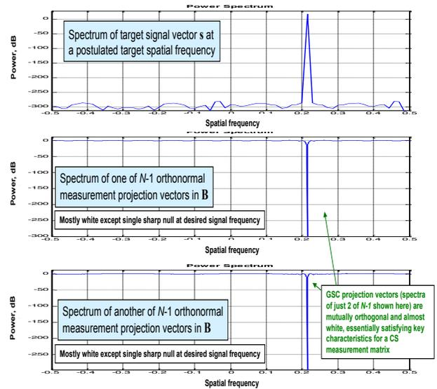
Figure 3. The top subfigure is the frequency response of the filter associated with the desired signal vector:  $\mathbf{s}$ . The bottom two subfigures are the frequency responses associated with two of the  $N-1$  auxiliary channel filters of the GSC. The spectra of the auxiliary filters are nearly 'white' aside from one very narrow null, representing a very good approximation to an ideal 'white' CS sampling function.
