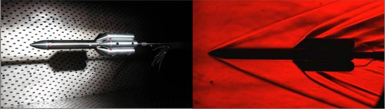
Dynetics wind tunnel testing of an SLV
